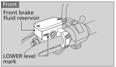
If the brake fluid level in either reservoir is below the LOWER level mark or the brake lever and pedal freeplay becomes excessive, inspect the brake pads for wear. If the brake pads are not worn, you most likely have a leak. Have your motorcycle inspected by your dealer.
