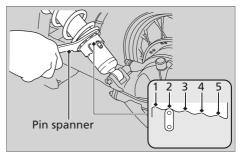
Attempting to adjust directly from 1 to 5 or 5 to 1 may damage the shock absorber.
