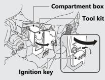
Insert the ignition key and turn it counterclockwise to unlock.
