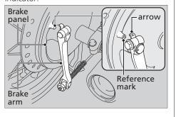
When the brake is applied, an arrow attached to the brake arm moves toward a reference mark on the brake panel. If the arrow aligns with the reference mark on full application of the brake, the brake shoes must be replaced.
