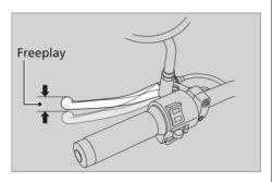
Check the clutch cable for kinks or signs of wear. If necessary have it replaced by your dealer.
