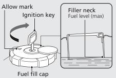
Do not fill with fuel above the filler neck. Fuel type: Unleaded gasoline only Recommended fuel octane number: Pump Octane Number (PON) 86 or higher. Tank capacity: 2.77 US gal (10.5 liters) Reserve capacity: 0.61 US gal (2.3 liters)
