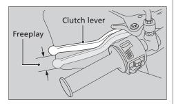
Check the clutch cable for kinks or signs of wear. If necessary have it replaced by your dealer.
