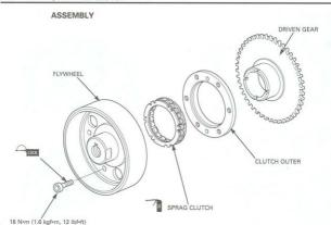
Apply engine oil to the sprag clutch contacting surfaces.
