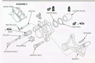
Coat the new piston seal with clean brake fluid. Coat the new dust seal with silicone grease.
