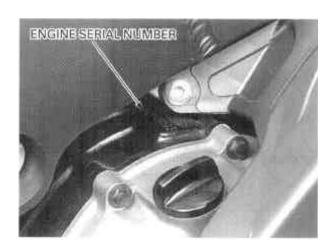
(2) The engine serial number is stamped on the right side of the upper crankcase.
