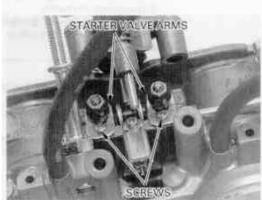
Install the wax unit assembly onto the throttle body, tighten the screws to the specified torque.
