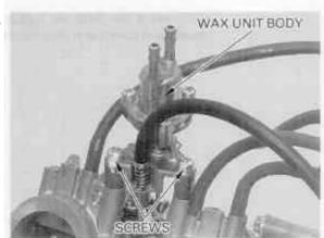
Turn the starter valve screw until it seats lightly, then back it out as noted during removal.
