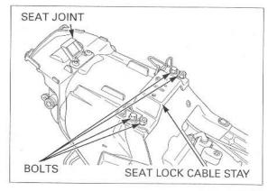
Disconnect the seat lock cable from the cable stay.
