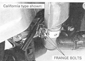
Remove the muffler mounting bolt and washer. Remove the muffler clamp bolt and nut.
