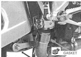
Temporarily install the exhaust pipe joint nuts, and mounting bolts/nut/washers.
