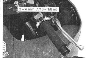
Throttle grip free play can be adjusted at either end of the throttle cable.
