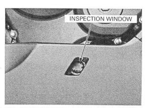
If the level is below the lower level line, remove the oil filler cap and fill the crankcase with the recommended oil up to the upper level line as following procedures.
