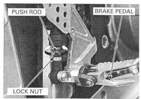
Make sure the push rod threads can be seen through the pedal joint hole.
