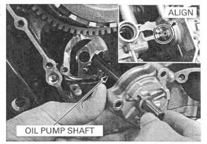
Install and tighten the three flange bolts securely.
