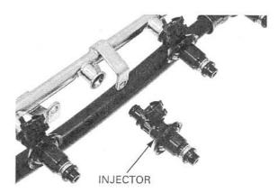
Remove the O-ring, seal ring, cushion ring and dust seal.
