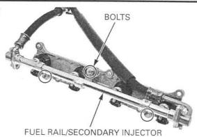
Remove the injectors from the fuel rail.
