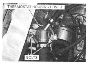
Remove the thermostat from the housing.
