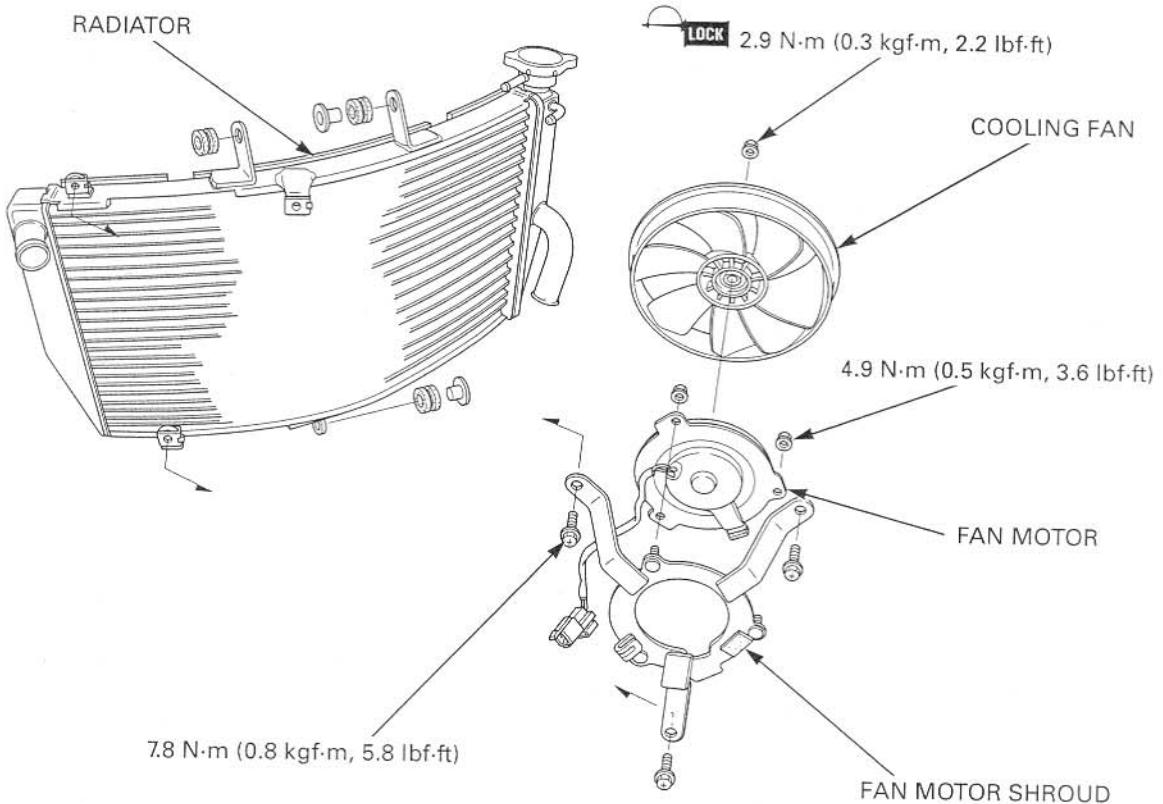
Install the fan motor onto the fan motor shroud and tighten the nuts to the specified torque.
