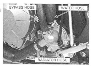
Remove the two SH bolts and clamp, two flange bolts with two sealing washers and water pump cover.
