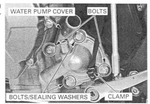
Connect the radiator hose, water hose and bypass hose, then tighten the clamp screws.
