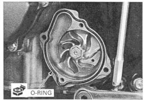
Install the water pump cover, new two sealing washers with two flange bolts and two SH bolts, clamp.
