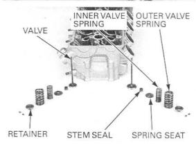
springs has a orange paint marks and the intake valve springs has blue paint marks.
