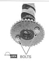
Exhaust camshaft Clean and apply a locking agent to the cam pulse only: generator rotor bolt threads.
