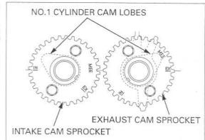
Clean and apply a locking agent to the cam sprocket bolt threads.
