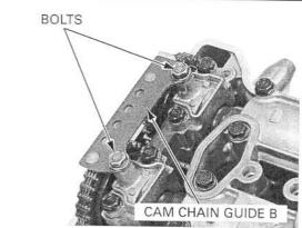
In case the cam sprockets were removed, tighten the cam sprocket bolts to the specified torque.
