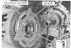
Apply molybdenum oil solution to the clutch outer guide sliding surface.
