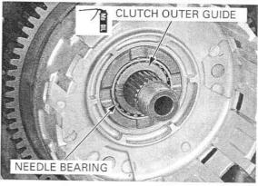
Install the thrust washer.
