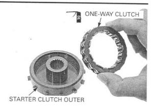
Install the snap ring into the starter clutch outer groove securely.
