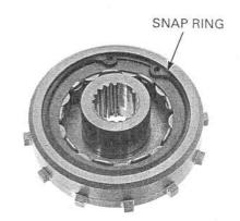
Install the starter driven gear and needle bearing into the starter clutch outer while turning the starter driven gear clockwise.
