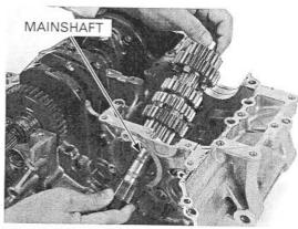
Install the bearing into the crankcase with the marked side facing out.
