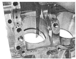
Measure the piston pin bore.
