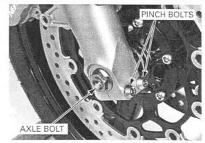
Loosen the left axle pinch bolts. Remove the axle and front wheel.
