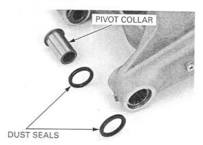
Remove the pivot collar and dust seals from the swingarm right side pivot.
