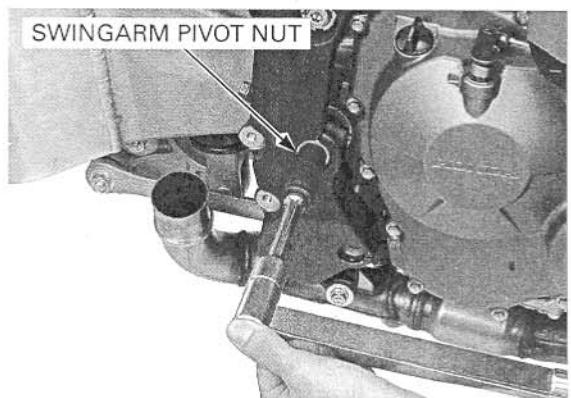
Tighten the right swingarm pivot pinch bolt to the specified torque.
