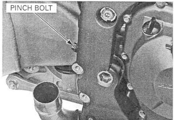
Tighten the left swingarm pivot pinch bolt to the specified torque.
