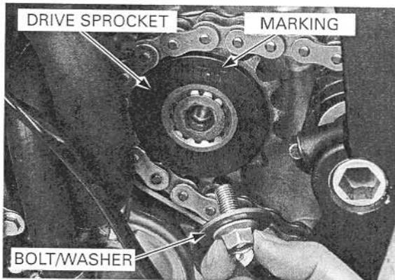
Install the spacer and drive sprocket cover, tighten the bolts securely.
