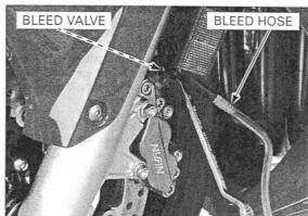
Loosen the bleed valve and pump the brake lever or pedal.
