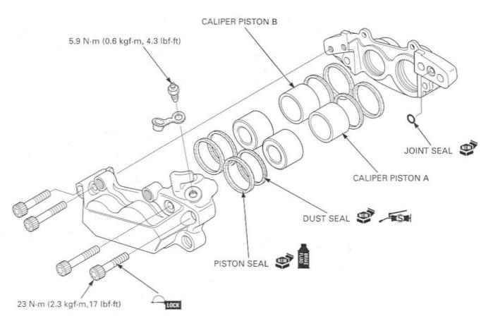
Coat new piston seals with clean brake fluid. Coat new dust seals with silicone grease.
