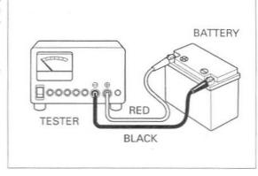
For accurate test results, be sure the tester's cables and clamps are in good working condition and that a secure connection can be made at the battery.
