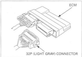
Connect the peak voltage tester or peak voltage adaptor probes to the connector terminal of the wire harness side.
