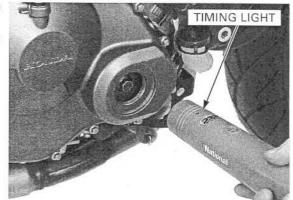
The ignition timing is correct if the index mark on the right crankcase cover aligns between the "F" mark and three punch marks on the ignition pulse generator rotor as shown.
