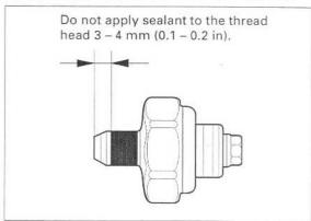
Install the oil pressure switch onto the switch base, tighten the oil pressure switch to the specified torque while holding the switch base.
