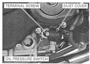
Apply sealant to the oil pressure switch threads as shown.
