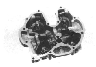
Set the 8 mm and 6 mm cylinder head cover bolts on the cylinder head cover.
