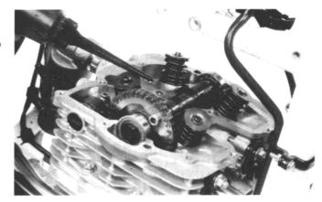
Turn the crankshaft until the cam lobes face down as shown. Install a new cylinder head cover gasket and dowel pin.
