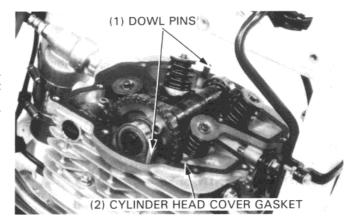
Clean the cylinder head mating surface of the cylinder head cover.
