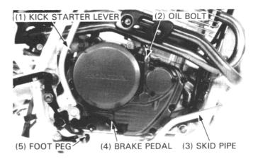
Remove the bolts and nuts holding the right crankcase cover and remove the cover.
