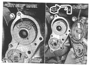
Install the oil filter cover and tighten the bolts to the specified torque.
