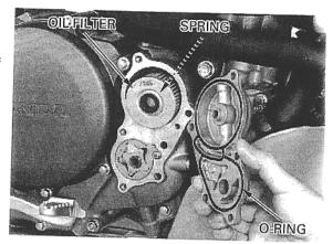
Apply engine oil to a new O-ring and install it to the oil filter cover.
