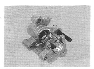
Measure the caliper piston O.D.
